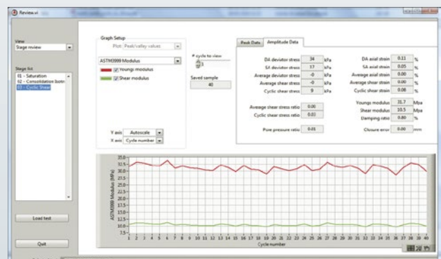
Young's and shear modulus are monitored during the cyclic stage.
