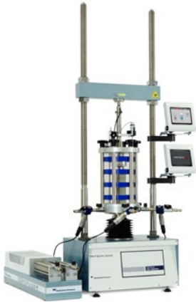
Configuration with automatic pressure/volume controller, HYDROMATIC STANDALONE
