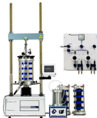
Configuration with Air/ water bladders and volume change device
