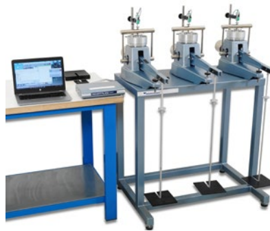
Electronic Configuration Displacement transducer and GEODATALOG8
